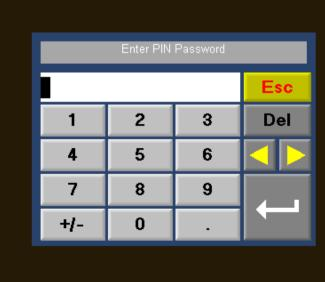
Enter the 4 digit Pin No & press the enter key (return arrow) to move onto the parameter set up pages
